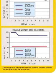
Racing Ignition Coil Test Data
