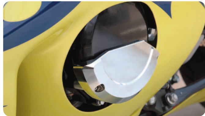
GSX1300R HAYABUSA(1999~ 2010) Machined Engine protector (shift pedal side)
